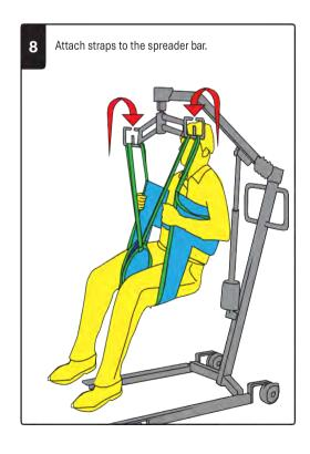
Before every lift visually examine the slings structural integrity. If there is any sign of excessive damage to the fabric or straps DO NOT USE THE SLING.
