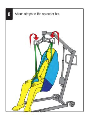
Before every lift visually examine the slings structural integrity. If there is any sign of excessive damage to the fabric or straps DO NOT USE THE SLING.
